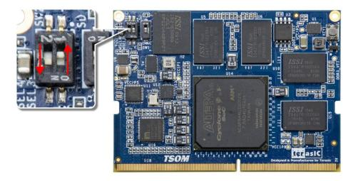
Figure 3-1 TsoM module is setting to FPPx32 mode
