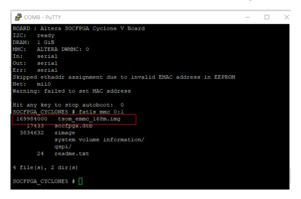
11. Enter the command "fatload mmc 0:1 \$loadaddr tsom\_emmc\_168M.img" to load the .img file into the DDR3.
