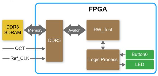
Figure 6-5 Block Diagram of the DDR3\_RTL Demonstration
