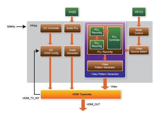
Figure 6-1 Block Diagram of the HDMI TX Demonstration
