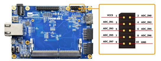
Figure 5-6 Signals of the 2x5 Header
