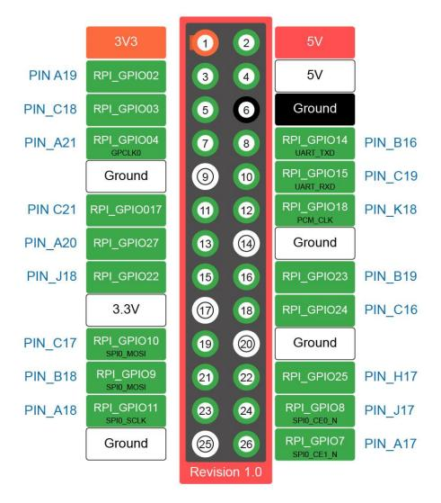
Figure 4-7 Raspbery Pi 2x13 expansion header
