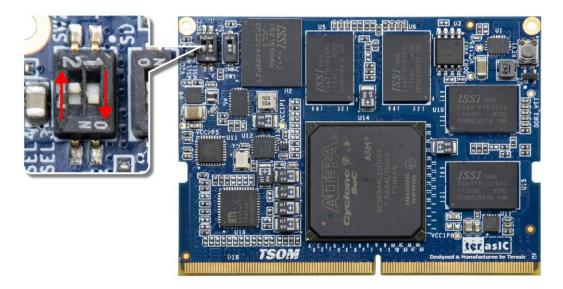
Figure 3-5 SW2 Setting Resistors (AS Mode)
