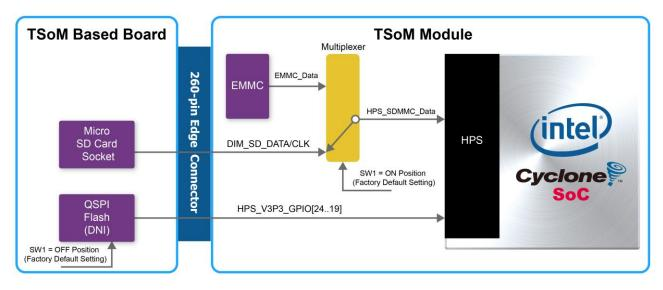
Figure 3-2 Boot device for HPS on the TsoM evaluation kit
