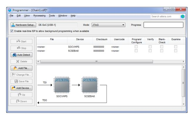
Figure 3-11 FPGA and HPS detected in Quartus programmer
