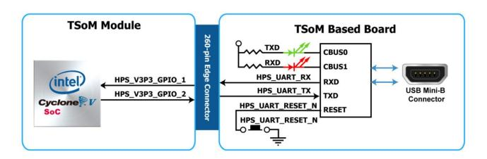
Figure 4-3 Connections between the HPS and FT232R Chip
