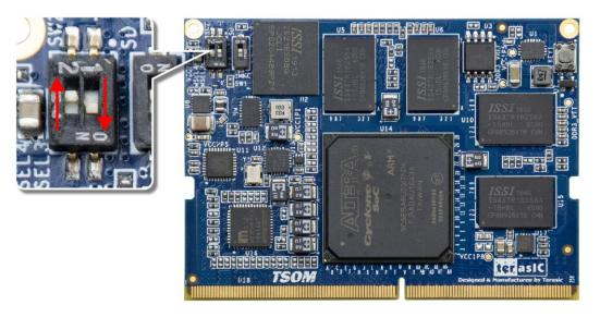
Figure 7-1 SW2 Setting Resistors (AS Mode)
