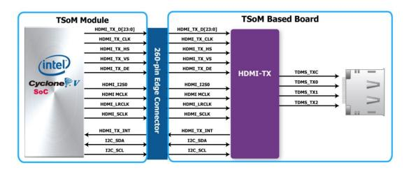
Figure 5-8 Connections between the Cyclone V SoC FPGA and HDMI Transmitter Chip
