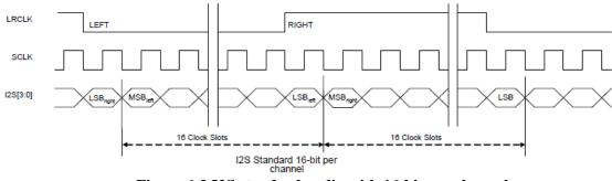
Figure 6-2 I2S standard audio with 16-bit per channel
