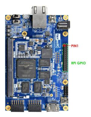
Figure 4-6 Raspbery Pi 2x13 expansion header
