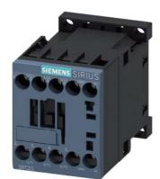
Power contactor, AC-3 12 A, 5.5 kW / 400 V 1 NO, 600 V AC, 60 Hz 3-pole, Size S00 screw terminal
