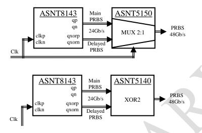
Fig. 2. PRBS Frequency Doubling
