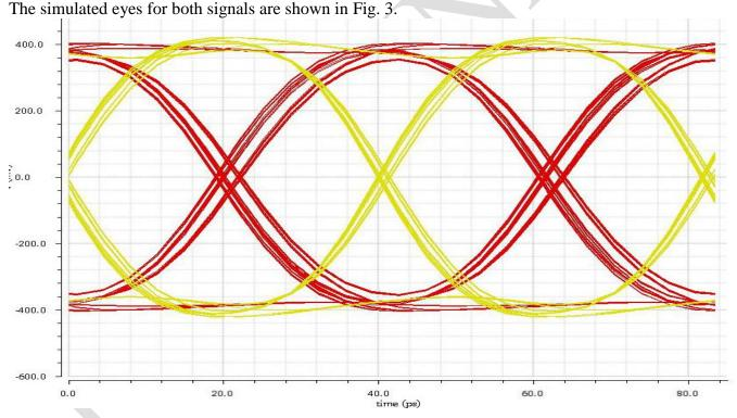
Fig. 3. 24Gbps PRBS Output Eye Diagram (Simulation, Slow Corner, 125°C)
