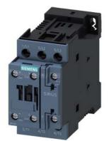
power contactor, AC-3 9 A, 4 kW / 400 V 1 NO + 1 NC, AC (50 / 60 Hz) DC operation 200-280 V AC/DC, 3-pole Size S0, screw terminal
