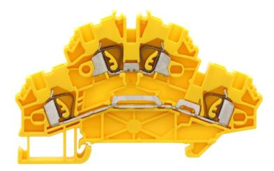
Double-level terminal, Tension-spring connection, Mounting type: Mounting rail TS 35/7.5, Rated cross-section: 2.5 mm<sup>2</sup>, Width: 5.1 mm, Colour: Yellow
