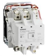
Mechanically held lighting contactor, Contactor amp rating 100A, 0 N.C. / 4 N.O. poles, 110VAC 50HZ/120VAC 60HZ coil, Non-combination type, Enclosure NEMA type (open), No enclosure
