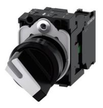
Selector switch, illuminable, 22 mm, round, plastic, white, selector switch, short, 2 switch positions O-I, latching, 10:30h/13:30h, with holder, 1 NO, screw terminal, with laser labeling, upper case and lower case, always upper case at the beginning of the word
