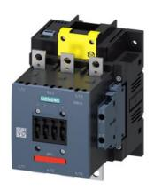
Contactor, AC-1, 275 A/690 V/40  $^{\circ}$ C, S6, 3-pole, 96-127 V AC/DC, F-PLC-IN with varistor, 2 NO+2 NC, permanently mounted, Connection rail/ screw terminal
