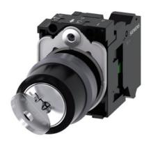
RONIS key-operated switch, 22 mm, round, plastic with metal front ring, lock number SB30, with 2 keys, 2 switch positions O-I, latching, actuating angle 90°, 10:30h/13:30h, key removal O+I, with holder, 1 NO, spring-type terminal, possible special locks: SB31, 421, 455, with laser labeling, lower case
