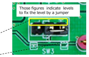
On this evaluation board, jumpers as shown in the picture above are provided for setting operation of TB67S103AFTG
