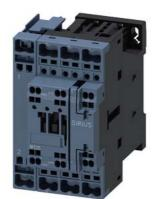
Power contactor, AC-3 25 A, 11 kW / 400 V 2 NO + 2 NC 24 V AC, 50 Hz 4-pole size S0 Spring-type terminals 1 NO + 1 NC integrated
