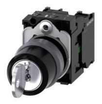
RONIS key-operated switch, 22 mm, round, plastic with metal front ring, lock number SB30, with 2 keys, 3 switch positions I-O-II, latching, actuating angle 2x45°, 10:30h/12h/13:30h, Key removal I+O+II, with holder, 1 NO, 1 NO, screw terminal, possible special locks: SB31, 421, 455, with laser labeling, inscription or symbol Customer-specific selection with SIRIUS ACT configurator (CIN)
