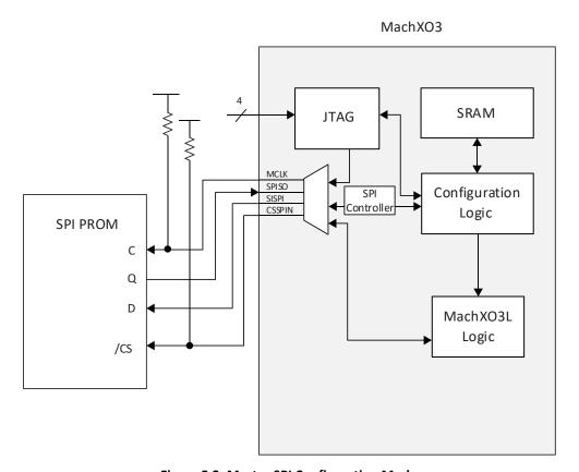
Figure 5.2. Master SPI Configuration Mode
