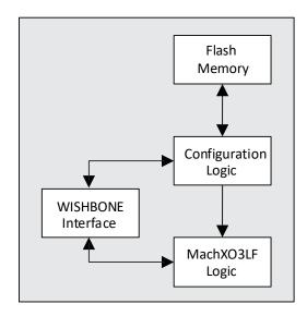
Figure 6.1. WISHBONE Configuration Mode
