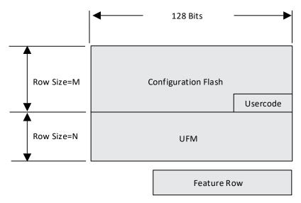
Figure 4.3. Flash Memory Space of a MachXO3LF Device
