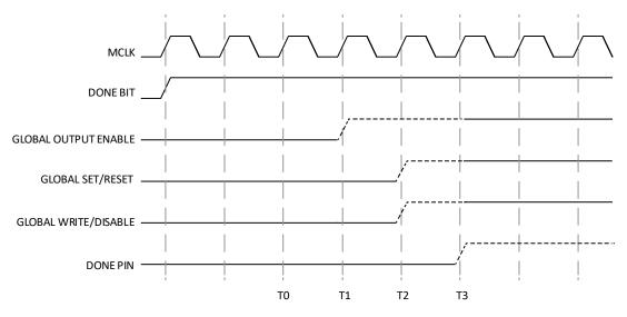
Figure 8.1. Wake-up Sequence Using Internal Clock
