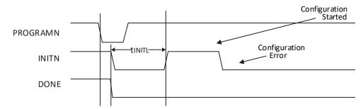
Figure 4.7. Configuration Error Notification
