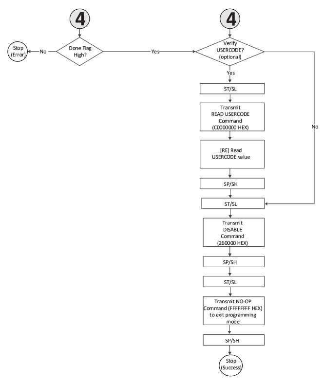
Figure 9.3. MachXO3 Slave SPI/I<sup>2</sup>C SRAM Configuration Flow
