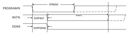
Figure 4.6. Configuration from PROGRAMN Timing
