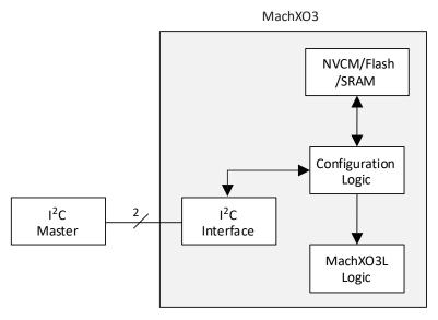
Figure 5.4. I<sup>2</sup>C Configuration Logic
