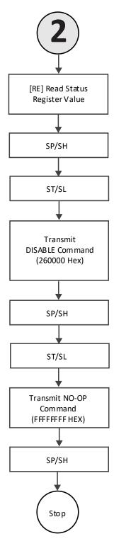
Figure 9.6. Slave SPI/I<sup>2</sup>C SRAM Read Status Register Flow
