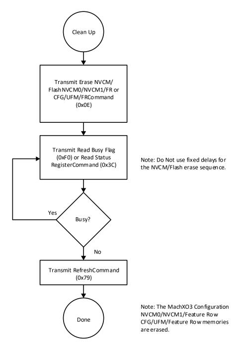
Figure 9.2. MachXO3 NVCM/Flash Memory Programming Flow
