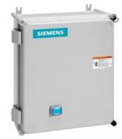
Reversing motor starter, Size 2 1/2, Three phase full voltage, Amb. compensate bimetal OLR, Contactor amp rating 60A, Non-combination type, Enclosure type 4X fiberglass, Water/dust tight noncorrosive
