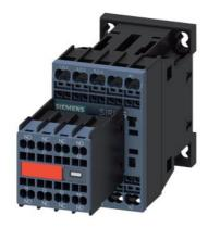
Power contactor, AC-3 7 A, 3 kW / 400 V 24 V DC 3-pole, Size S00 Spring type terminal Captive auxiliary switch
