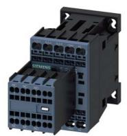
Power contactor, AC-3 9 A, 4 kW / 400 V 2 NO + 2 NC, 110 V AC, 50 / 60 Hz, 3-pole, Size S00, Spring-type terminal Removable auxiliary switch
