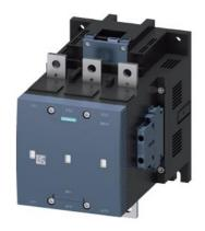
vacuum contactor, AC-3 400 A, 200 kW / 400 V AC (50-60 Hz) / DC operation 21-27.3 V AC/DC auxiliary contacts 2 NO + 2 NC 3-pole, frame size S12 busbar connections drive: electronic with SPS interface DV 24 V
