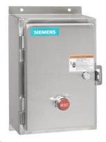
Non-reversing motor starter, Size 2 1/2, Single phase, 2-pole, Amb compensate bimetal OLrelay Contactor amp rating 60Amp 190 220/220 240V 50/60HZ coil, Non-combination type, Enclosure type 4X 304 S-steel, Water/dust tight noncorrosive
