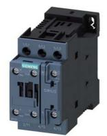
power contactor, AC-3 9 A, 4 kW / 400 V 1 NO + 1 NC, 60 V DC 3-pole, Size S0 screw terminal
