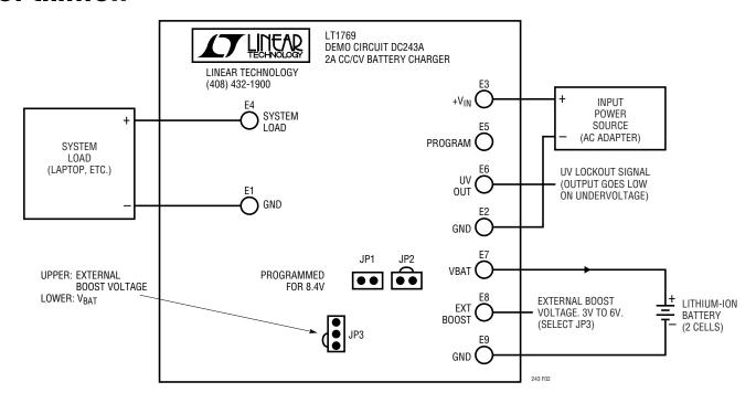
Figure 3. Demo Board Wiring Diagram
