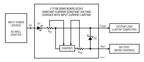
Figure 2. Simplified Block Diagram of Demo Board
