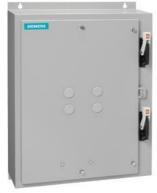
Duplex starter w/o alternator, Size 1, Three phase full voltage, Amb. compensate bimetal OLR, contactor A rating 27A, 110V 50Hz / 120V 60Hz coil, Combination type, Two 3A circuit breakers, Enc NEMA type 4 painted steel, Water/dust tight for outdoors
