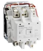
Mechanically held lighting contactor, Contactor amp rating 100A, 0 N.C. / 5 N.O. poles, 110VAC 50HZ/120VAC 60HZ coil, Non-combination type, Enclosure NEMA type (open), No enclosure
