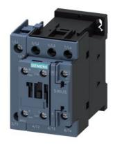
Contactor, AC-1, 35 A/400 V/40 °C, S0, 4-pole, 24 V AC, 50/60 Hz, 1 NO+1 NC, screw terminal
