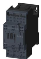
power contactor, AC-3 12 A, 5.5 kW / 400 V 1 NO + 1 NC, 110 V AC 50 / 60 Hz, 3-pole Size S0, Spring-type terminal
