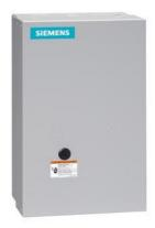
2-speed 3-phase motor starter, Size 4, Two separate windings, Constant or variable torque, Solid-state overload relays, Low Spd OLR range 50-200A, High Spd OLR range 50-200A, 110V 50Hz / 120V 60Hz coil, Enclosure NEMA type 1, Indoor general purpose use
