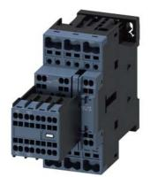
power contactor, AC-3 9 A, 4 kW / 400 V 2 NO + 2 NC, 110 V AC 50 / 60 Hz, 3-pole Size S0, Spring-type terminal Removable auxiliary switch
