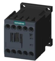
Power contactor, AC-3 16 A, 7.5 kW / 400 V 1 NC, 48 V AC, 50/60 Hz 3-pole, Size S00 screw terminals
