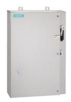
Non-reversing motor starter, Size 4, Three phase full voltage, Solid-state overload relay, OLR amp range 50-200A, Combination type, 150A circuit breaker, Encl NEMA type 4X 304 S-Steel, Water/dust tight noncorrosive, Standard width enclosure
