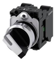
Selector switch, illuminable, 22 mm, round, metal, shiny, white, selector switch, short, 2 switch positions O-I, latching, actuating angle 90°, 10:30h/13:30h, with holder, 1 NO, 1 NC, spring-type terminal, Z=20-unit packaging
