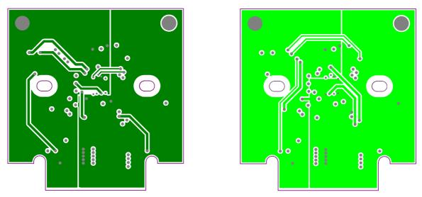
Figure 4: epc635 Card Edge Connector Carrier: Layout middle top and bottom
