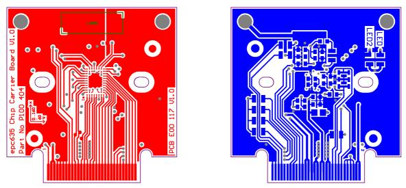
Figure 3: epc635 Card Edge Connector Carrier: Layout top and bottom
