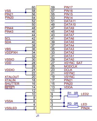
Figure 7: Pin table card edge connector J1
