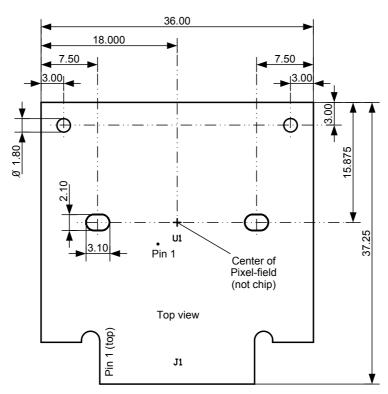
PCB material: Glass epoxy FR-4, thickness 1.6mm
