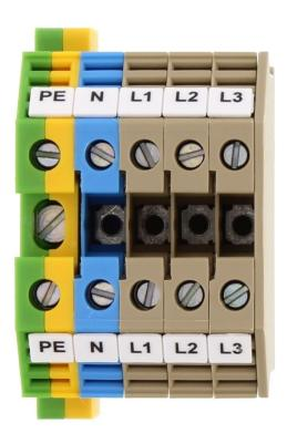
Five-wire mains-connection block, Screw connection, Mounting type:Mounting rail TS 35/7.5 and TS 32, Rated cross-section: 4 mm², Colour: Multi-coloured
