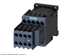
Power contactor, AC-3 9 A, 4 kW / 400 V 3 NO + 2 NC, 240 V AC 50 / 60 Hz, 3-pole, Size S00, screw terminal Varistor plugged on
