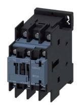
power contactor, AC-3 12 A, 5.5 kW / 400 V 1 NO + 1 NC, 400 V AC, 50 Hz 400-440 V, 60 Hz, 3-pole Size S0 ring cable lug connection
