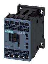
power contactor, AC-3 12 A,  $5.5\,kW$  / 400 V 1 NC, 24 V DC 0.7-1.25\*US with integrated diode, 3-pole size S00, spring-type terminal suitable for PLC outputs not expandable with auxiliary switch
