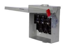
Siemens Low Voltage Circuit Protection Heavy Duty Safety Switches. Type: ENCLOSED, SAFETY SWITCH Std: UL V. Rating: 240V A. Rating: 200A Wattage: 3W No. Of Poles: 2P F. Rating: 60Hz Action: DOUBLE THROW Material: 304SS Enclosure: TYPE 3R. 2-3 point mounting holes. O. Cycles: 8000 O. Temperature: (-20F-120F) AMBIENT TEMPERATURE Environmental Conditions: OUTDOOR
