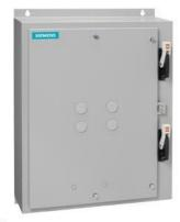
Duplex starter w/o alternator Size 1 Three phase full voltage Solid-state overload relay OLR amp range 0.25-1A 240VAC 50Hz / 277VAC 60Hz Coil Combination type Two 30A disconnect switches Encl NEMA type 4X 304 S. Steel Water/dust tight non-corrosive
