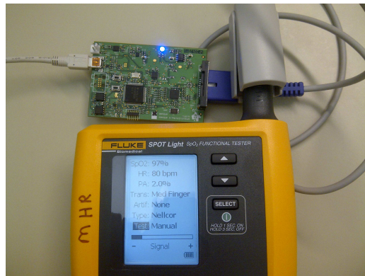
Figure 35. Fluke SPOT Light SpO2 Functional Tester Setup
