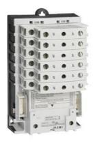
Electrically held lighting contactor, (convertible to mech. held), Amp rating 30A (tungsten 20A), 7 N.C. / 2 N.O. poles, 575-600V 60Hz/550V 50Hz coil, Non-combination type, Enclosure NEMA type (open), No enclosure
