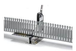
Hand lever is ergonomically designed to reduce user fatigue. Measuring guide incorporates both imperial and metric values which eliminates the need for secondary measurement devices.
