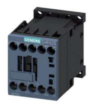
Power contactor, AC-3 16 A, 7.5 kW / 400 V 1 NO, 24 V AC, 50/60 Hz 3-pole, Size S00 screw terminals
