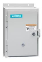
Reversing motor starter, Size 1, Three phase full voltage, Solid-state overload relay, OLR amp range 5.5-22A, 24VAC 50-60Hz coil, Non-combination type, Enclosure type 12, Dust/drip proof for indoors, Standard width enclosure
