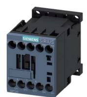
Power contactor, AC-3 7 A, 3 kW / 400 V 1 NC, 24 V DC with varistor integrated, 3-pole, Size S00, screw terminal
