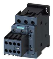
Power contactor, AC-3 32 A, 15 kW / 400 V 2 NO + 2 NC, 24 V AC 50/60 Hz, 3-pole Size S0, screw terminals Removable auxiliary switch
