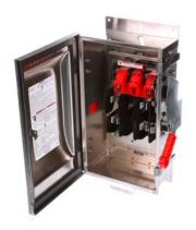
Siemens Low Voltage Circuit Protection Heavy Duty Safety Switches. Type: ENCLOSED, SAFETY SWITCH Std: CSA V. Rating: 240V A. Rating: 60A Wattage: 3W No. Of Poles: 3P F. Rating: 60Hz Action: SINGLE THROW Material: SS Enclosure: TYPE 4X. 2-3 point mounting holes. Insulation: YES O. Cycles: 10000 O. Temperature: (-20F-120F) AMBIENT TEMPERATURE Environmental Conditions: INDUSTRIAL CORROSIVE RESISTANCE
