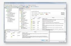
Analyze your design easily by filtering out messages once you have checked them. Messages can be filtered individually, by IDs, categories, or severity.
