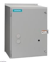
Electrically held lighting contactor, Contactor amp rating 400A, 0 N.C. / 3 N.O. Poles, 110VAC 50HZ/120VAC 60HZ coil, Non-combination type, (no disconnect device), Encl NEMA type 4X 304 S-Steel, Water/dust tight noncorrosive
