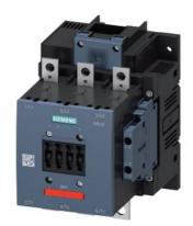
power contactor, AC-3 185 A, 90 kW / 400 V AC (50-60 Hz) / DC operation 23-26 V AC/DC auxiliary contacts 2 NO + 2 NC lateral, permanently mounted 3-pole, frame size S6 busbar connections drive: conventional
