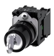
RONIS key-operated switch, 22 mm, round, plastic, lock number SB30, with 2 keys, 3 switch positions I-O-II, latching, 10:30h/12h/13:30h, Key removal I+O+II, with holder, 1 NO, 1 NO, screw terminal, possible special locks: SB31, 421, 455, with laser labeling, lower case
