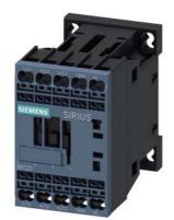
Power contactor, AC-3 7 A, 3 kW / 400 V 1 NO, 48 V AC 50 / 60 Hz, 3-pole, Size S00, Spring-type terminal
