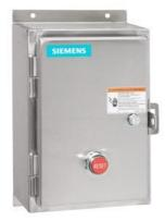
Non-reversing motor starter, Size 0, Single phase full voltage, Solid-state overload relay, OLR amp range 3-12A, 110V 50Hz / 120V 60Hz coil, Non-combination type, Encl. type 4X 304 S. Steel, Water/dust tight noncorrosive, Standard width enclosure
